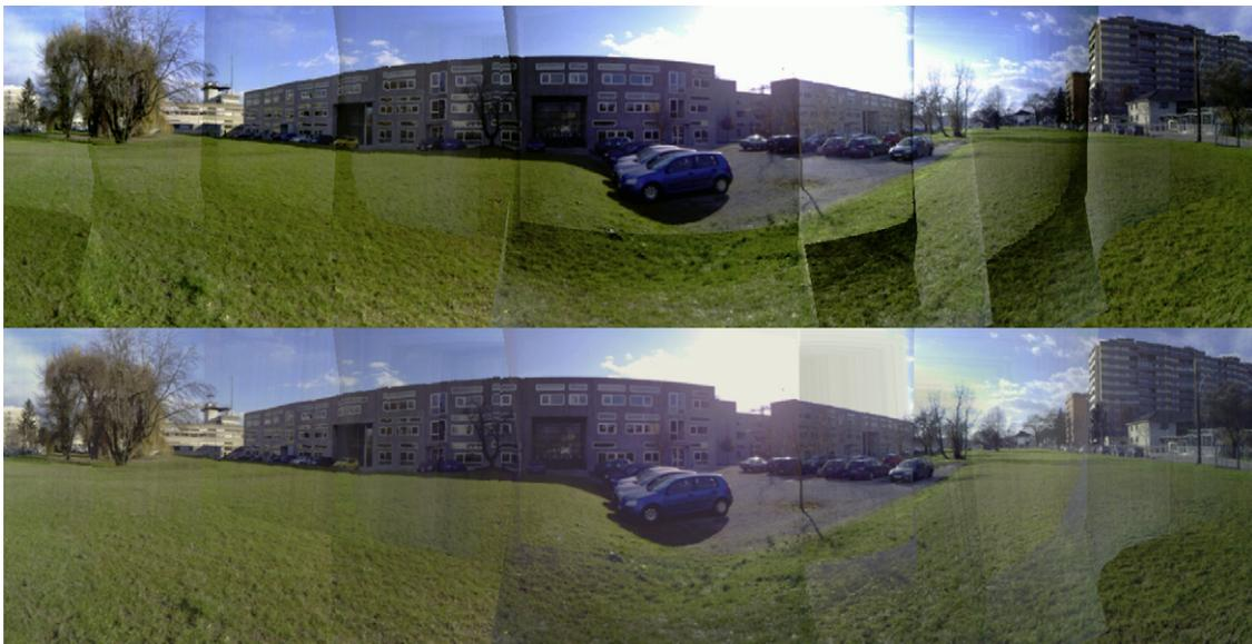
**Fig. 3.** (Top) A panorama image containing visual artefacts, which are caused by the automatic and continuous exposure adjustment of current mobile phone cameras. (Bottom) A panorama image that was created by extending the dynamic range during the mapping into the panorama and applying a tone-mapping afterwards.
