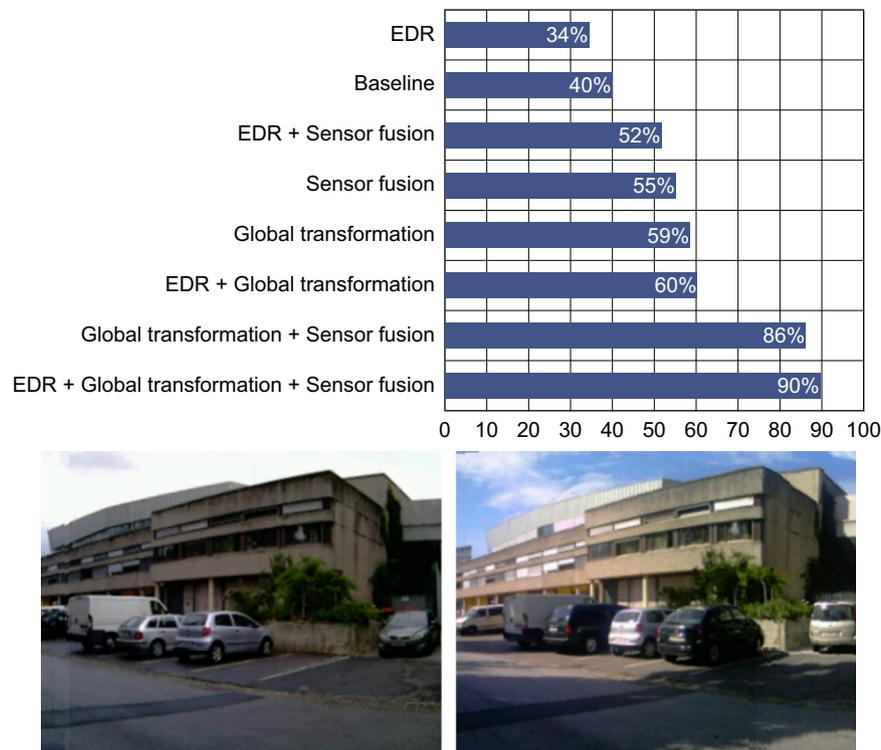
**Fig. 7.** Re-detection evaluation. (Top) Overview of the re-detection results. (Bottom) Fragments of two panorama images showing different environment conditions during the evaluation.
