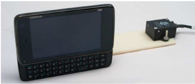
Fig. 6. The Nokia N900 used in our study with InterSense InertiaCube3 attached. The InertiaCube3 was attached at a distance to avoid magnetic disturbances from the device.
