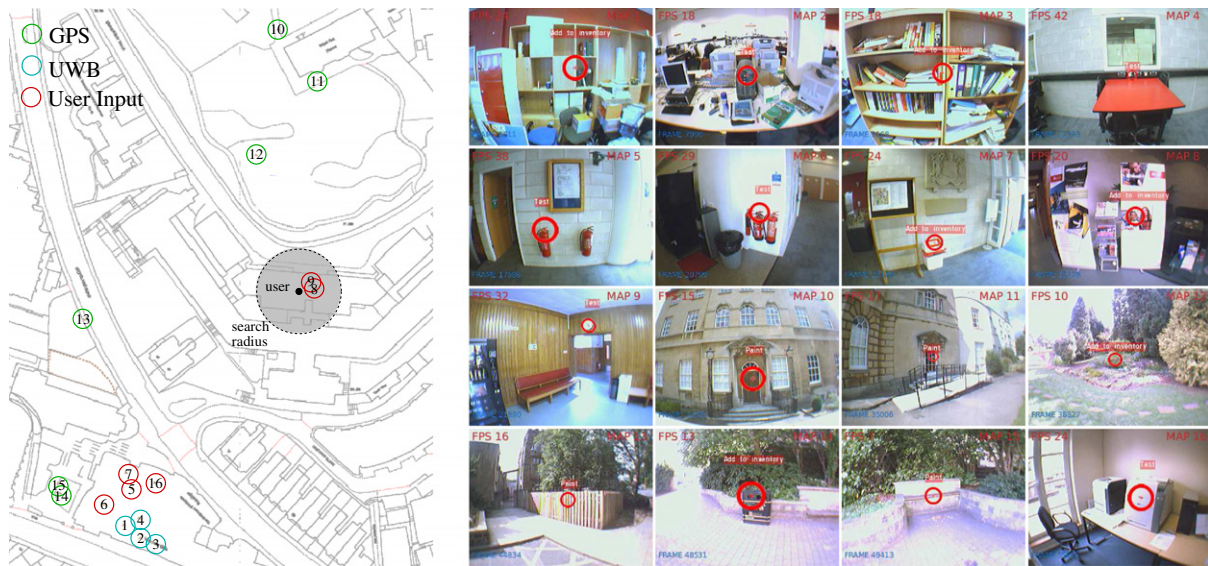
Fig. 13. An example of a global map generated by the ToMAR system. Sixteen local maps were created over an area of 0.1 km 2 containing a mixture of indoor and outdoor locations and with a mixture of GPS, UWB and User Input positioning. The 20 m search radius reflects that the user is currently in an area with no GPS or UWB coverage and is using interactive input positioning.
